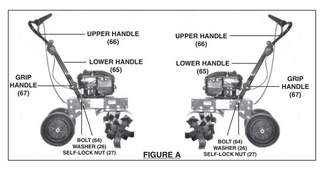
2. The Upper Handle (66) is folded for shipping purposes. Loosen the Grip Handles (67) located on each side of the Upper Handle. Unfold the Upper Handle to its normal working position. Then, firmly retighten each Grip Handle to secure the Upper Handle in place. (See Figure A.)
